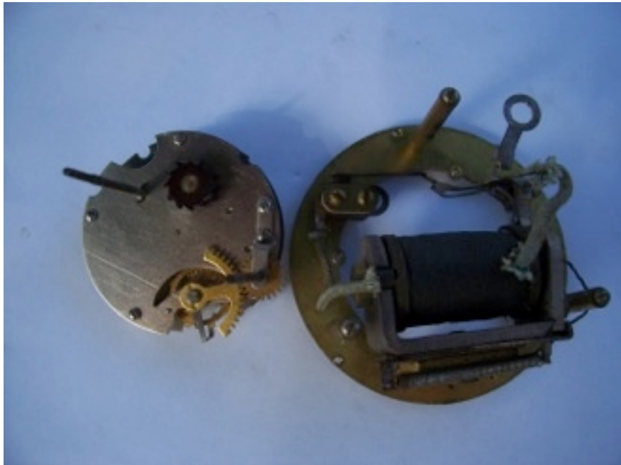
Clockworks removed from winder
