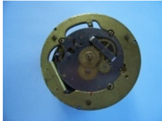
Front showing clockworks mounted in winder subassembly
